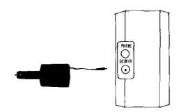
**Note:** When you connect the adapter, the DX-440 automatically disconnects the internal batteries.
